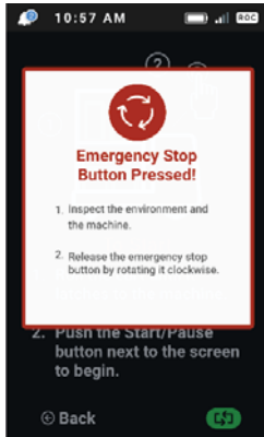
Figure 77: Emergency Stop button pressed
